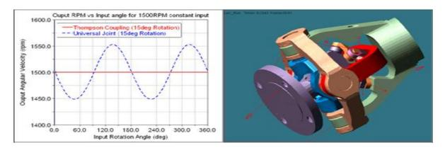
The graph above illustrates the difference in output motion of a universal joint (non-constant velocity) and a Thompson Coupling showing true constant velocity. The resultant non-constant velocity motion in traditional couplings produces shaft vibration and additional driveline forces causing increased wear and reliability issues for the power system.
