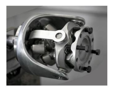
The TCVJ-2000-15 model shown has a customized 9 stud flange as required by the customer.
