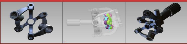
Graphic of the Thompson Coupling showing the internationally patented, spherical 4-bar linkage centring mechanism.
