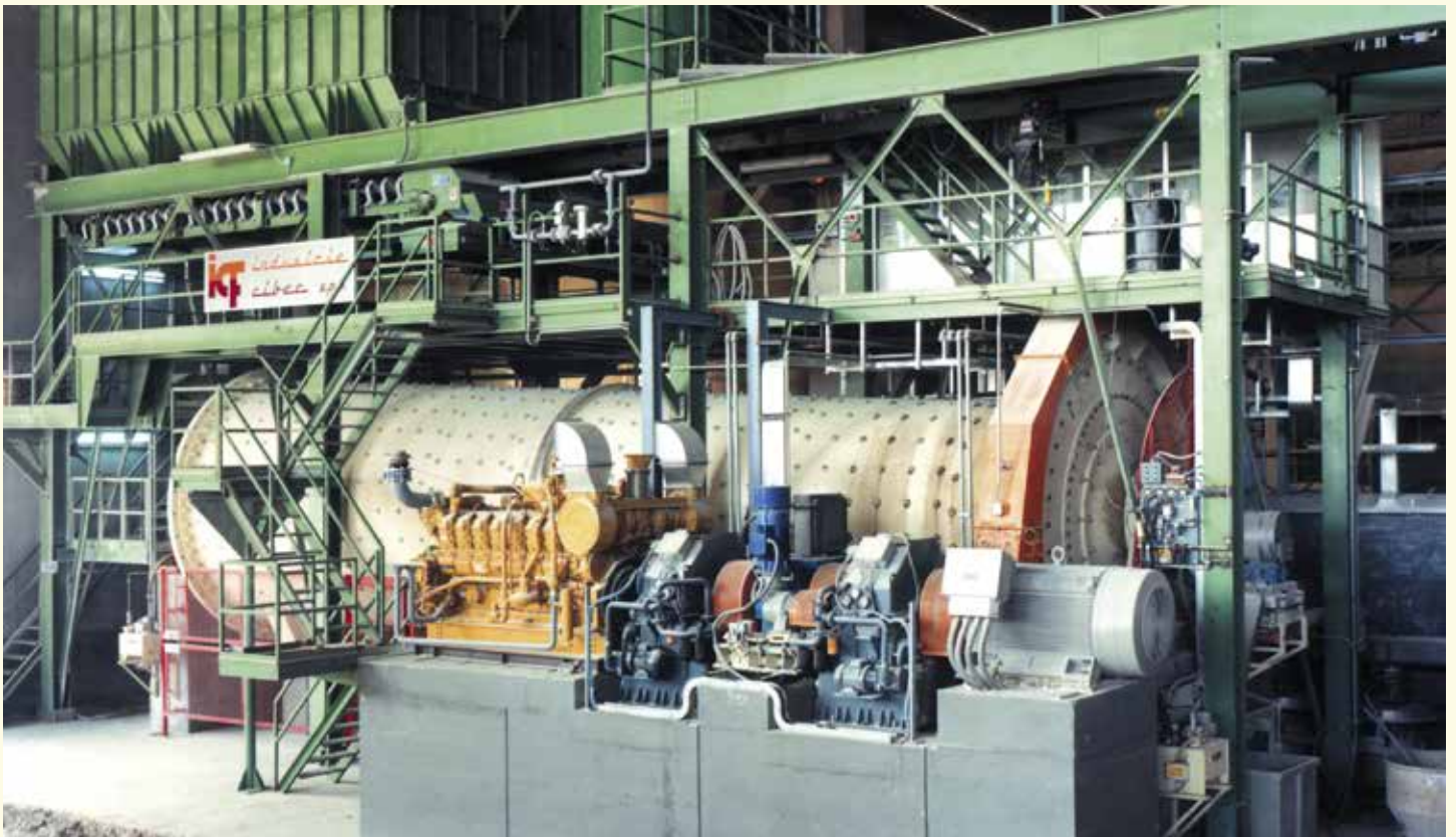
2x 34 KSL, 630 kW - 1000 rpm, Ceramic mill (Italy)
