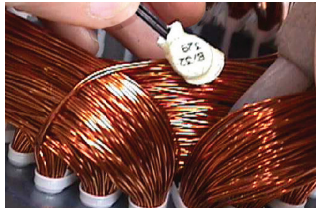
Figure 7.6 - Thermostat installation in the winding
