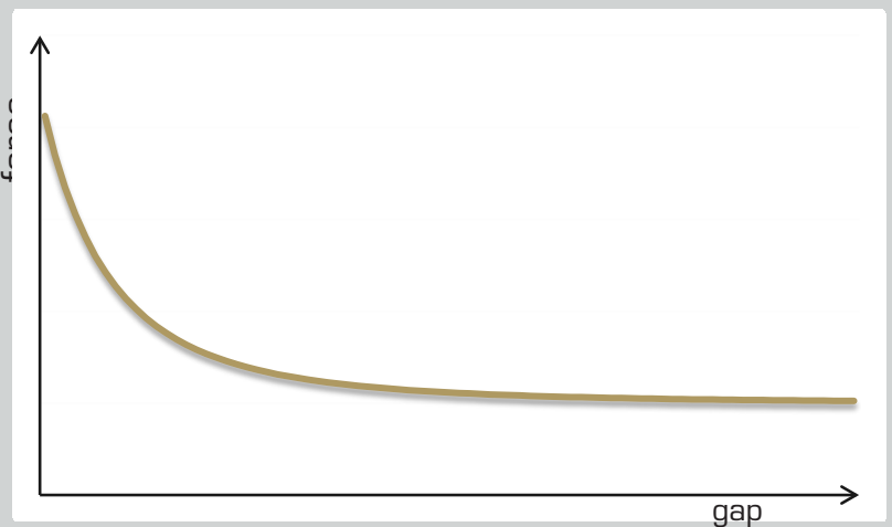
Magnetic force across the size of the air gap
