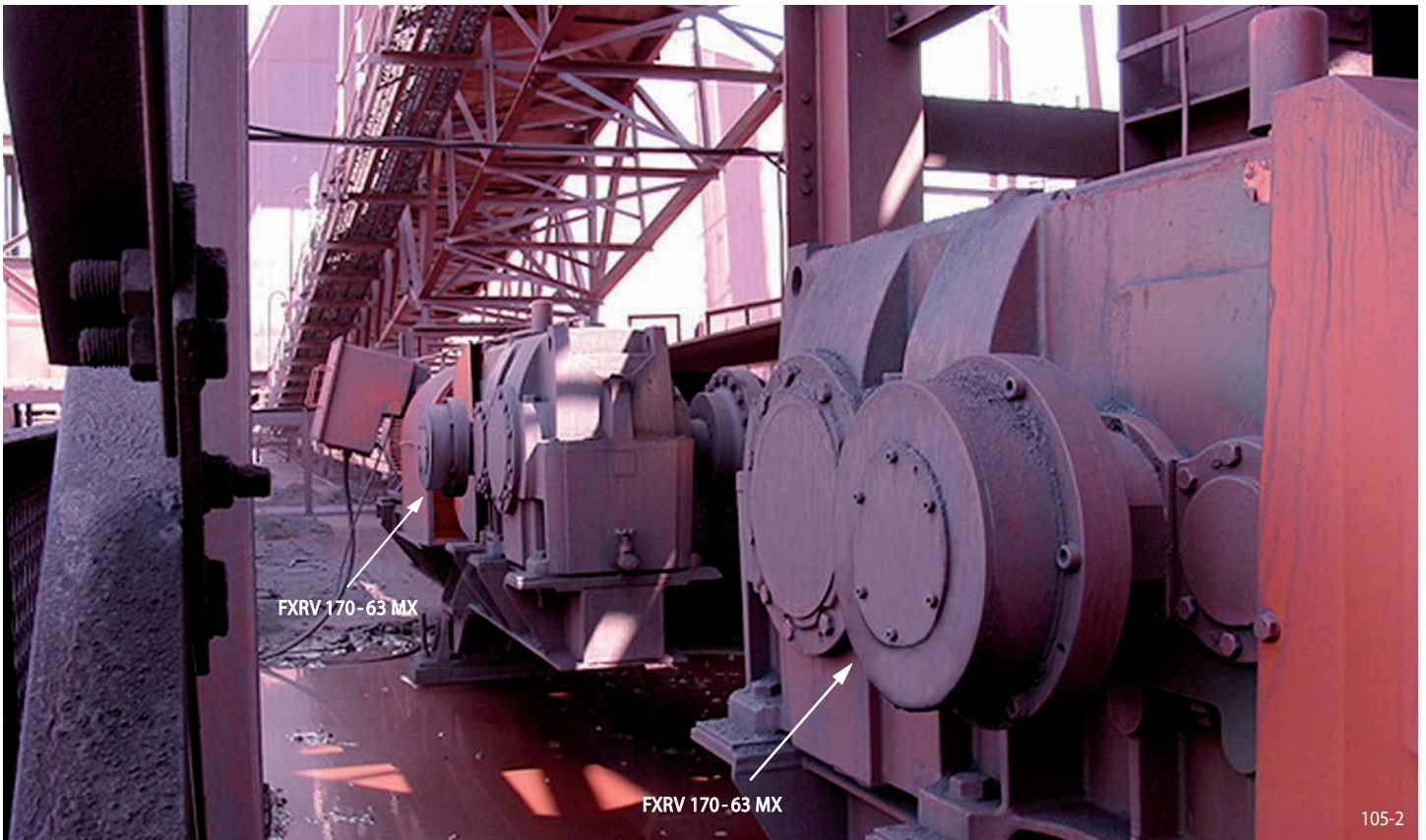
Iron ore conveyor plant in South Africa driven by three gear reducers with RINGSPANN backstops FXRV 170-63 MX.
