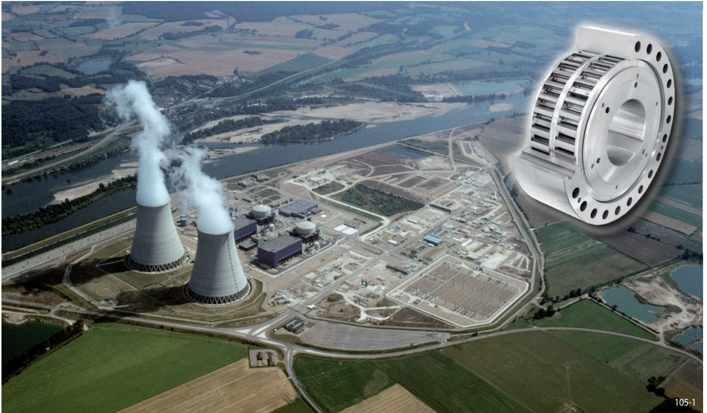
Backstop FXM 2.410 - 100 LX for the primary cooling water pump in a nuclear power station. Maximum torque 500 000 Nm. Speed 1 485 min -1 . In service since 1996. Manufactured and tested with extensive documentation from RINGSPANN GmbH, Bad Homburg.
