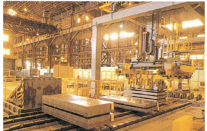
Steel panel conveyor
