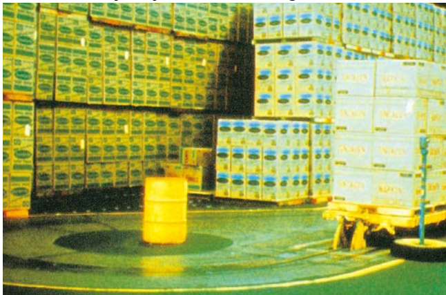
Towline conveyor system for stocking
