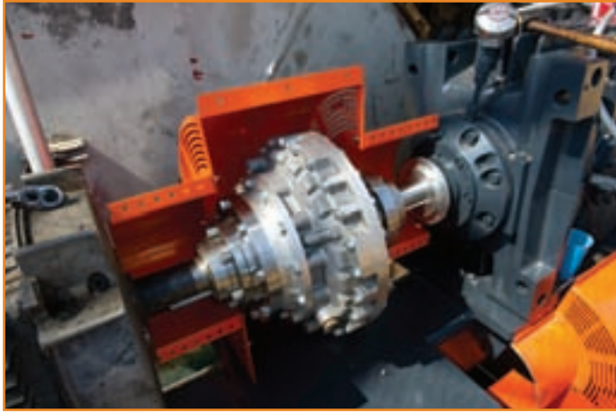
The new Falk V-Class drive is mounted with other drivetrain components that include a 100 hp motor and a Falk fluid coupling, protected by a Falk Orange Peel® guard.
