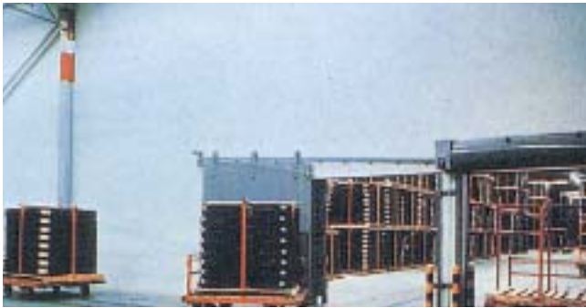
Towline conveyor system for tires
