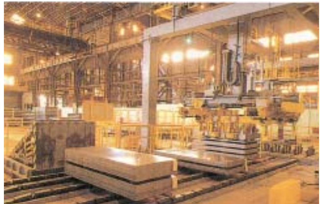
Steel panel conveyor
